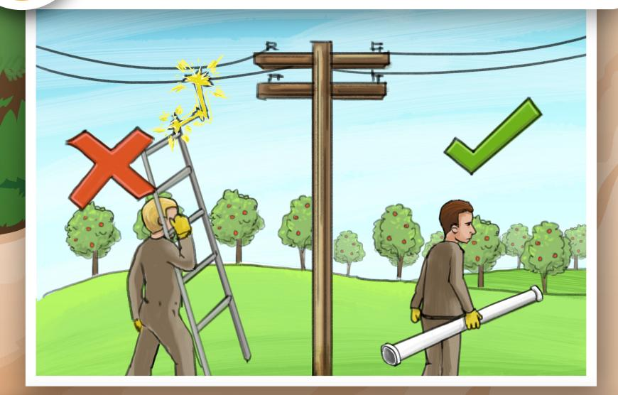
Lower equipment apparatus before driving.
